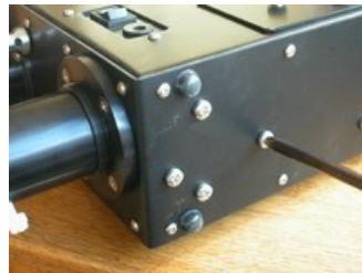
Main mirror adjusting screw
